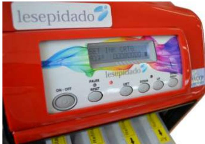
Remove cartridges/maintenance tank from their slot.
