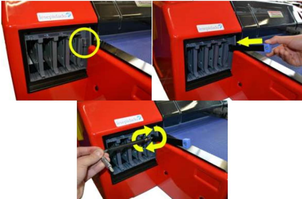
Remove each ink cartridge from its packaging. Lift both ink levers.
